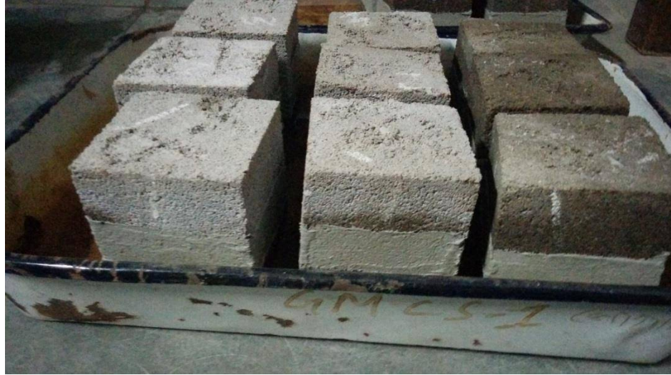
Fig 3.7 cubes arranged for sorptivity test
